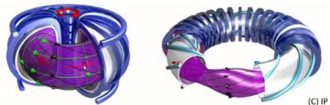
Figure 1.8. Schematic representation of a tokamak (left) and stellarator (right) [25].
