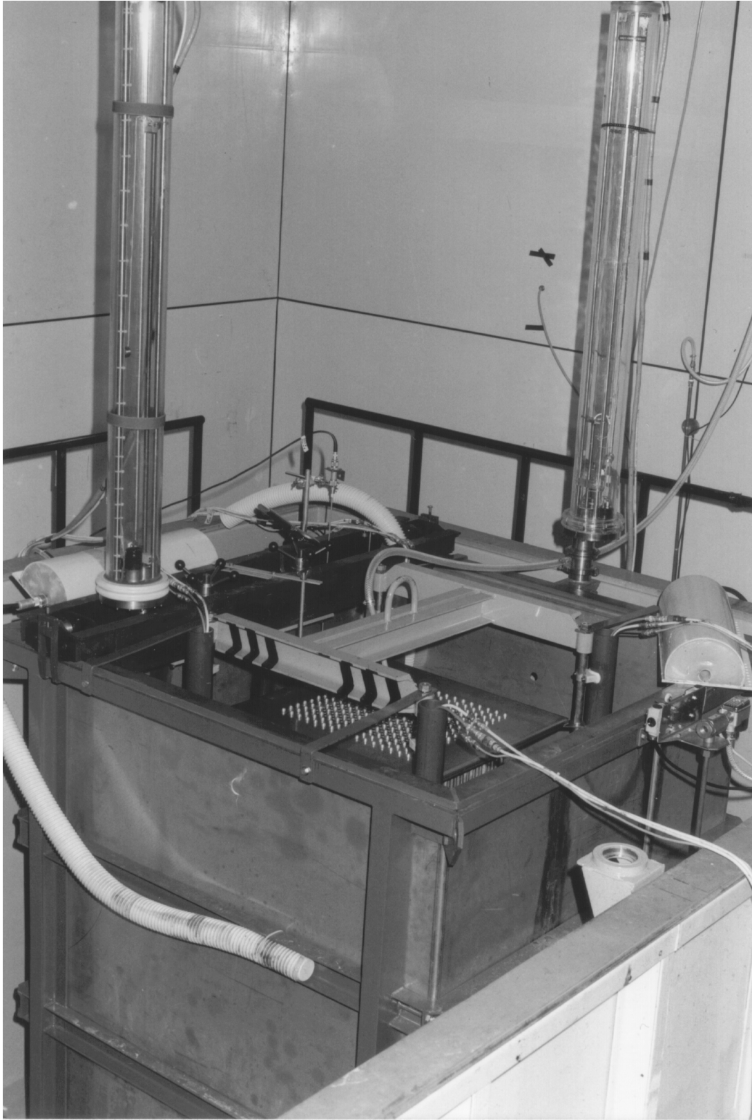
Figure 21: A photo of the experimental setup of LEU-COMP-THERM-039 series. A complete array of fuel rods is visible, while the experiments had different configurations of rods removed.
