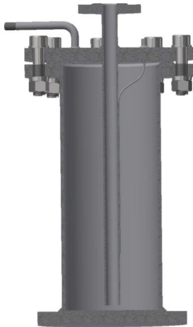
Figure 23: Main tank cross-section with visible gas inlet, lead outlet and thermocouple channel
