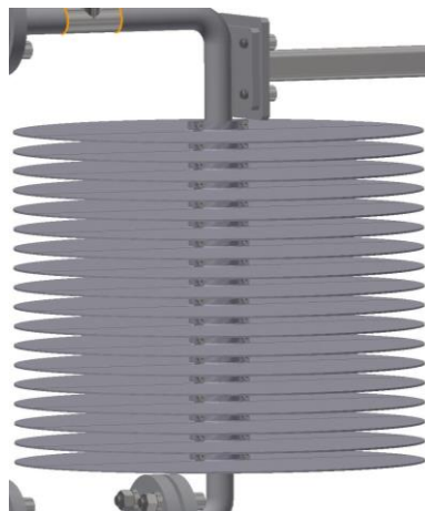
Figure 25: Heat radiator with adjustable fins
