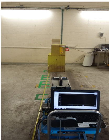
(a) Gamma spectrometry setup for measurement of waste. The maximum contact dose rate of the presented waste is 400 \mu\text{Sv/h} . In order to obtain a dead time below 10%, the distance detector-waste is set at 3 meters.
