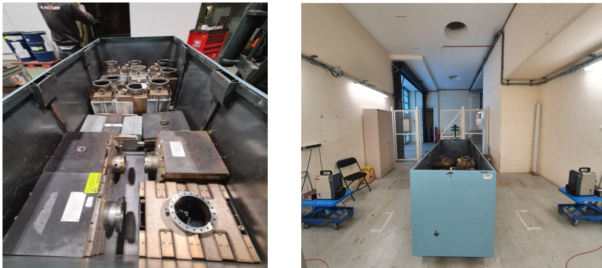
Figure 5.12: A 2.7 \text{ m}^3 container filled with 18 ion pumps (During filling up and measuring, respectively).
