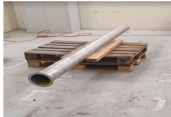
(b) Pipe with length > 2 meters and thickness 2 mm. The average dose rate for selected pipes is from 60 to 150 \mu\text{Sv/h} .
