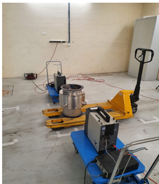
Figure 4.1: Gamma spectrometry setup for In-Toto measurement of the bulky pipe CR-015901.
