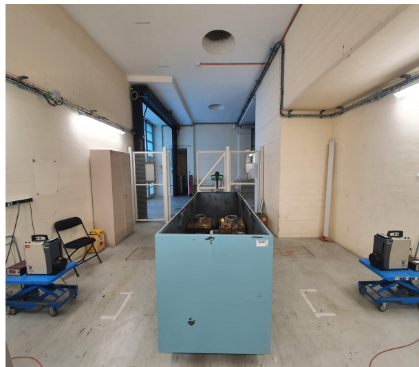
(b) Gamma spectrometry setup for measurement of container filled with ion pumps. The maximum contact dose rate of the container is above 250 \mu\text{Sv/h} . Due to space limitation, the maximum distance detector-waste is about 1.5 meters resulting in dead time of 24 %.
