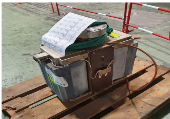
(c) Ion pump made of metallic non-magnetic and magnetic materials. The highest dose rate measured is < 1 \text{ mSv/h}
