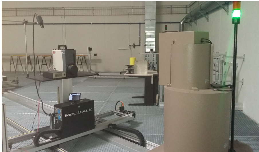
Figure 3.10: The interior of the Calibration Hall. Measurements performed using the Falcon 5000 detector. The measurements are fully driven from the control room, for dose exposure optimization and reduction.
